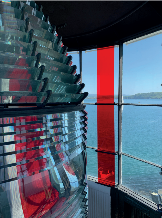
Views of the original optical apparatus. Unlike the situation in some other lighthouses, there are no rotating parts of the light mechanism. The optic remains in a fixed position and the light is switched on and off by electronic control.
